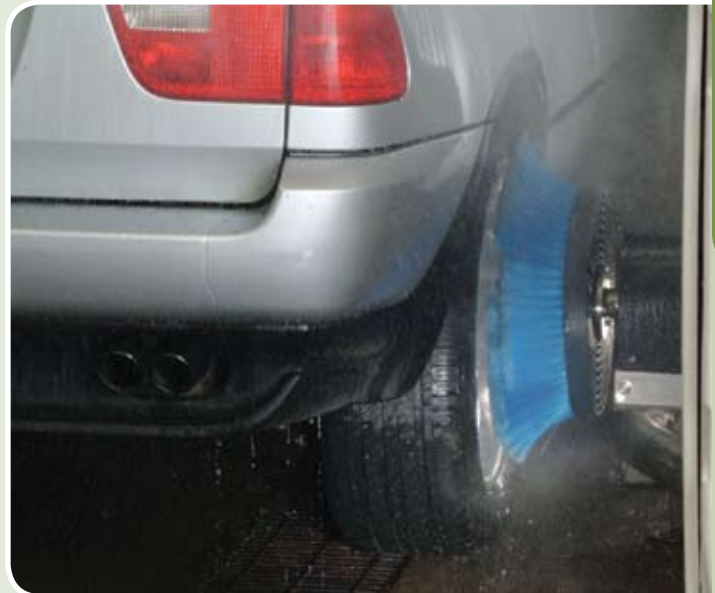
HubScrub ® wheel cleaning system reaches deep into convoluted wheel surfaces to remove stubborn road grime.
